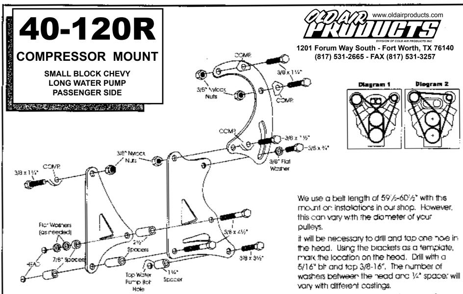
When using both A.C. and Alternator Brackets, belts can be run either of two ways, - as shown. They will require the use of 2 groove arank and water pump pulleys. Routing the belts as shown in Diagram 2 - will allow clearance for small blowers and extra room for I.P.I. air cleaners. The long belt will be approximately 71-72."
