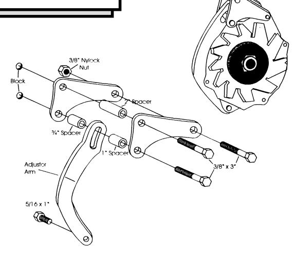
207 L- Alternator Mount - Small Block Chevy - Short Water Pump - Driver Side - Lower
