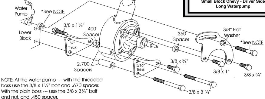
If your pump has a stud at the lower rear pivot point, remove it and use the 11/4" bolt and .400 spacer.
