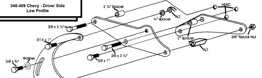
This bracket was designed to be used with Chevrolet double groove crank and water pump pulleys. The current G.M. part Numbers are 3744043 for the crank and 3995642 for the water pump.
