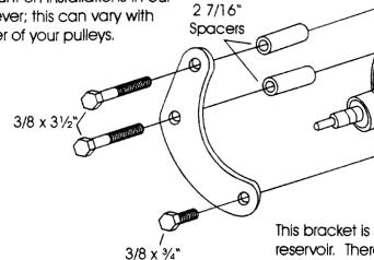
www.oldairproducts.com 1201 Forum Wav South - Fort Worth, TX 76140 (817) 531-2665 - FAX (817) 531-3257 **ENGINE** 3/8 x 1" 3/8" Flat Washer 3/8 x 1" 3/8" Flat .150 Washer NOTE: Some early blocks may have Spacer casting flash that will interfere with the rear of bracket. This is easily removed with a small grinding stone or hand file.
