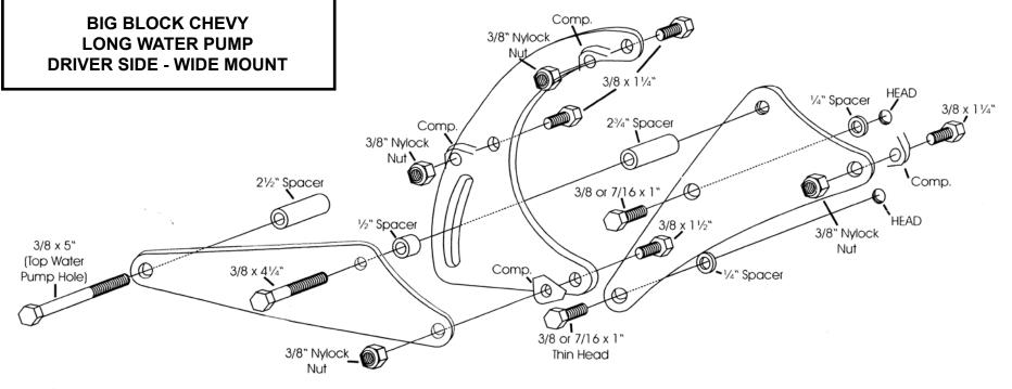
NOTE: Some heads have 3/8" bolt holes and some have 7/16". This kit includes both sizes of bolts for these holes.
