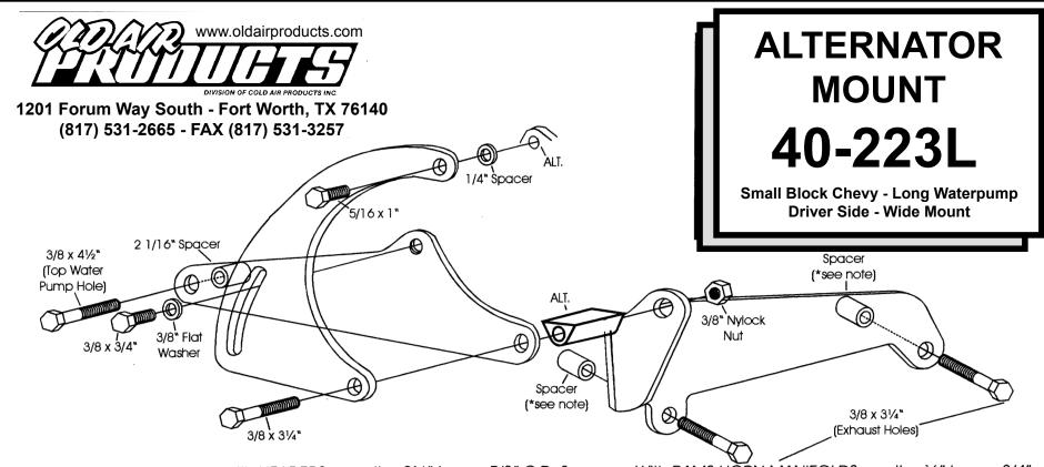
\*NOTE: Exhaust Spacers - with HEADERS - use the  $2\frac{1}{4}$ " long x 5/8" O.D. Spacers. With RAMS HORN MANIFOLDS use the  $\frac{1}{4}$ " long x 3/4" O.D. Spacer at rear hole of bracket and a  $1\frac{1}{16}$ " long x 3/4" O.D. Spacer at front hole of bracket. With the later DROP-TYP MANIFOLDS use the  $1\frac{1}{16}$ " long x 3/4" O.D. Spacers at both bracket holes. As with any mount system, assemble all of the brackets to engine BEFORE tightening the bolts.
