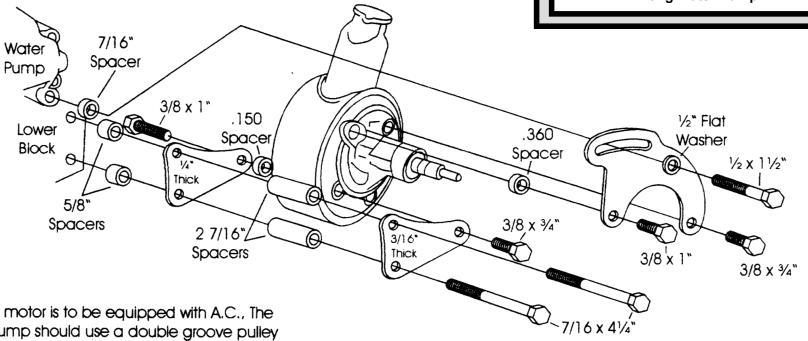
If the motor is to be equipped with A.C., The P.S. Pump should use a double groove pulley and the crankshaft a triple groove pulley. This will allow the use of a belt on the inner grooves of both the crankshaft and the power steering pump.
