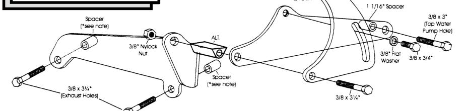
We use a belt length of 57-58" with this mount on installations in our shop. However; this can vary with the diameter of your pulleys.
