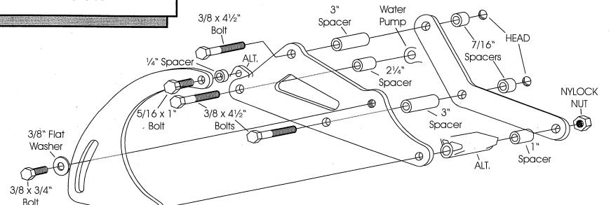
The alternator belt will run in the second grooves from the front of the crank and water pump pulleys originally used for the factory compressor. It was designed to be used with our Passenger Side Compressor Mount.
