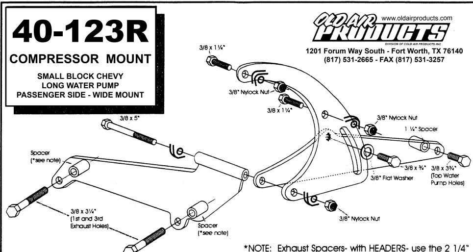
The compressor bett will run in the outer grooves of the crank and water pump pulleys originally used for the factory alternator. It was designed to be used with our 223L Driver's Side Alternator Mount.
